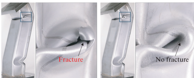
(a) 980 MPa Conventional DP (b) 980 MPa JEFORMA ™ Type 2
