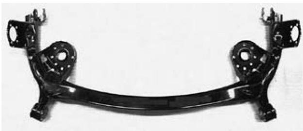
Photo 2 Rear axle to which the developed steel tube for torsion beam is applied
