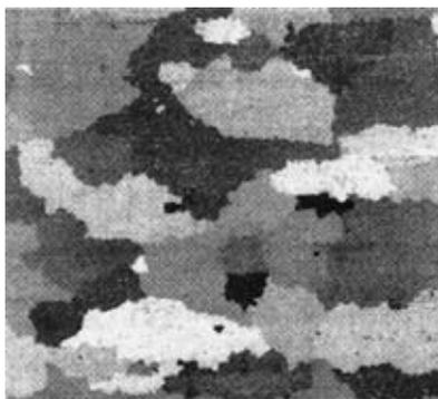
Photo 1 Typical macrostructure of grain oriented electrical steel
