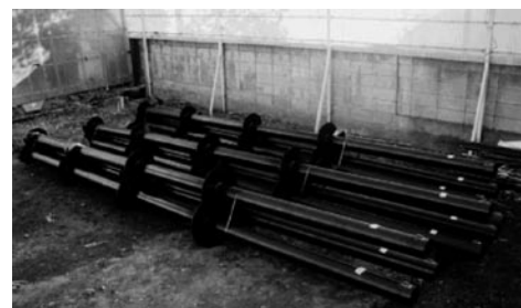
Photo 4 Screw pile, "micro-pile with plural wings"
