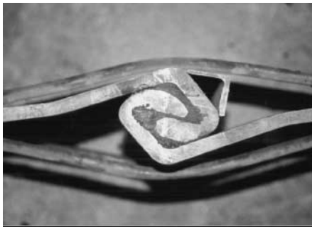
Photo 5 Steel sheet pile joints with polymer seals swelled with water
