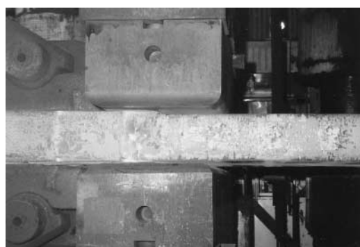
Photo 1 Forging reduction in thickness of CC slab
