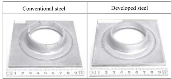
Photo 3 Hole expanded test piece (S35C)
