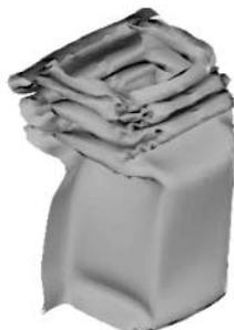
Fig. 18 Result of numerical crash simulation of hat square column
