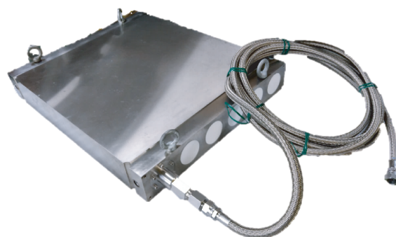
Photo 1 20 MN slab type load cell
