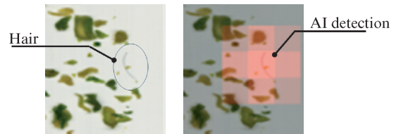
Fig. 2 Example of foreign object (hair) detection by AI
