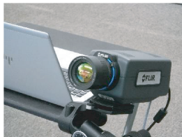
Photo 1 Airflow visualization system using infrared camera 3)
