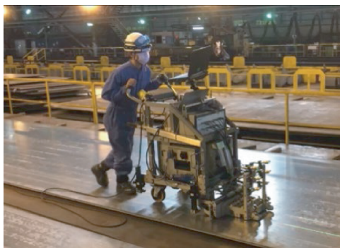
Photo 1 Surface hardness inspection
