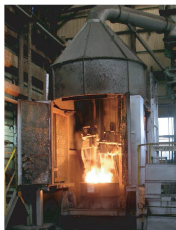
Photo 1 Reduction of MnO 2 by electric arc furnace
