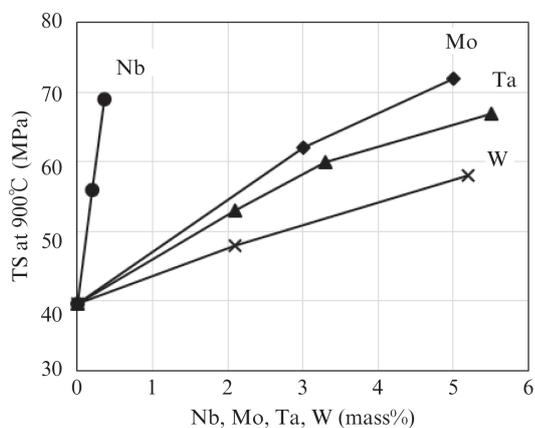
Fig. 5 Effect of additive elements on high-temperature strength of 20Cr-5Al Steel
