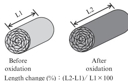
Fig. 4 Evaluation method of length change after oxidation test
