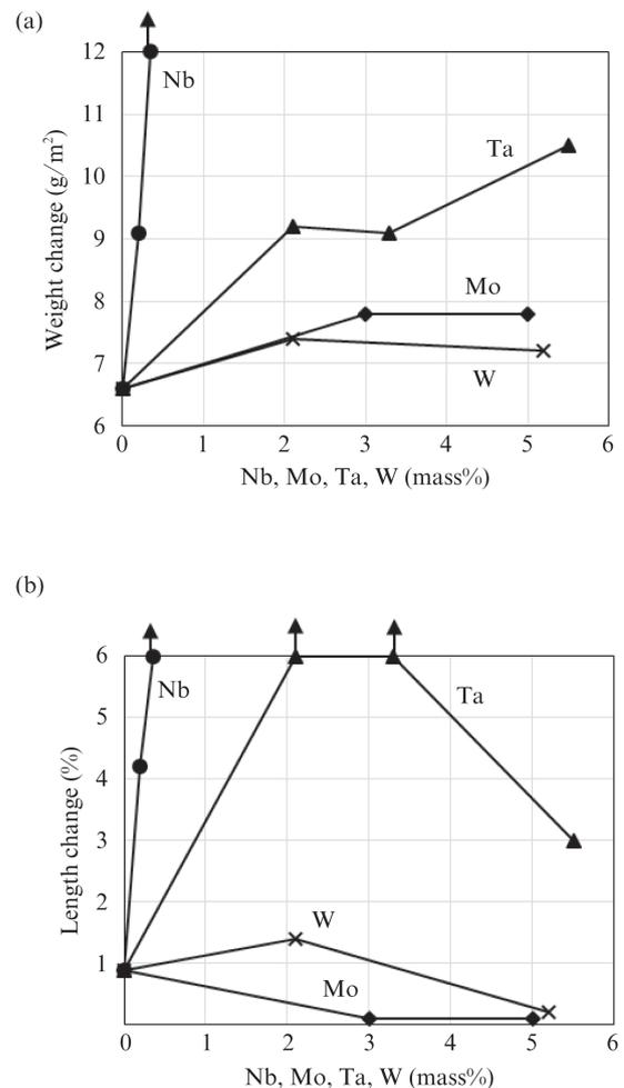
Fig. 6 Effect of additive elements on (a) weight change and (b) length change of 20Cr-5Al steel after 400 h oxidation at  $1\ 100^\circ\text{C}$
