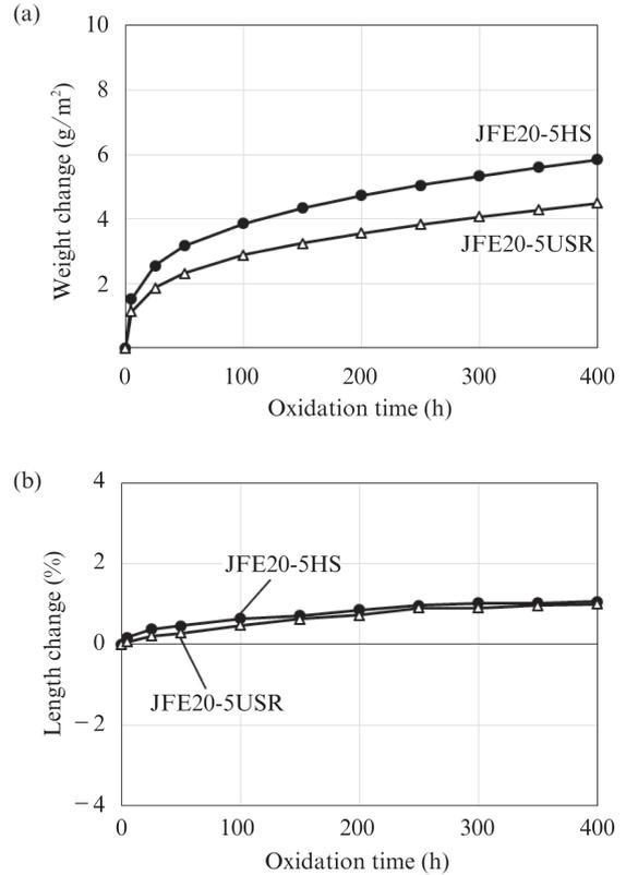
Fig. 11 Oxidation behavior of conventional steel and developed steel at 1100°C (40 μm thickness, BA)
