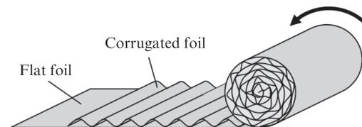
Fig. 3 Preparation method of test piece for oxidation test
