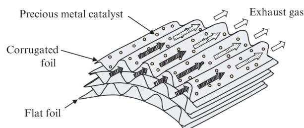
Fig. 2 Schematic of metal honeycomb system
