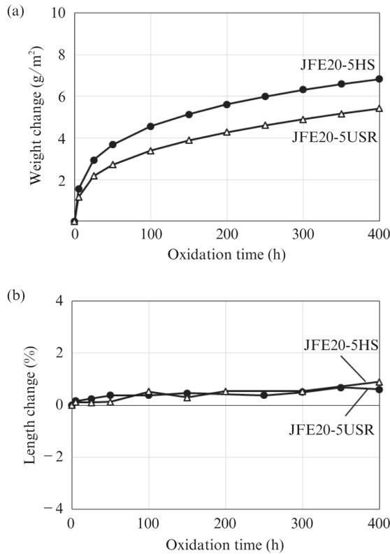
Fig. 10 Oxidation behavior of conventional steel and developed steel at 1100°C (40 μm thickness, HARD)
