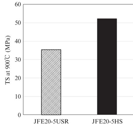
Fig. 9 High-temperature strength of conventional steel and developed steel
