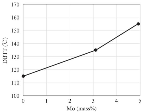
Fig. 8 Effect of Mo on ductile-brittle transition temperature of hot-rolled 20Cr-5Al steel
