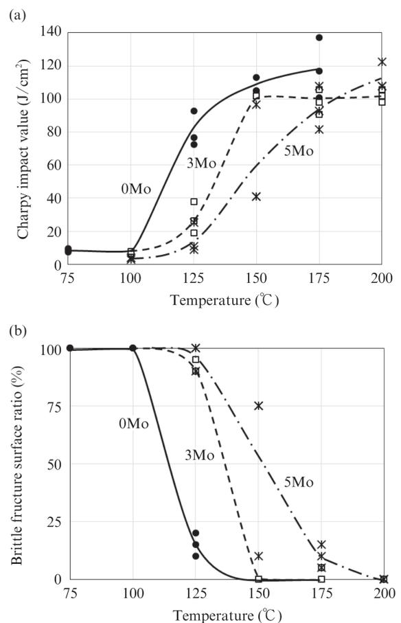
Fig. 7 Charpy impact test results of 20Cr-5Al-(0~5) Mo steel (a) Charpy impact value (b) Brittle fracture surface ratio
