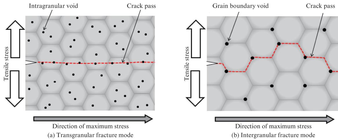
Fig. 7 Schematic diagram of fracture model of polycrystal MnZn ferrite
