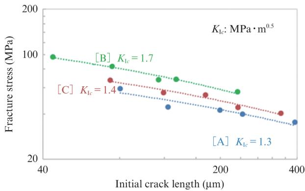
Fig. 5 Evaluation of fracture toughness by BI method
