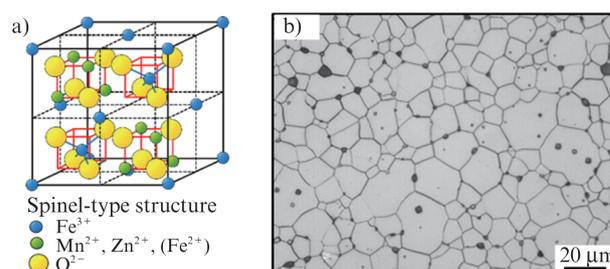
Fig. 1 Crystal structure and microstructure of MnZn ferrite
