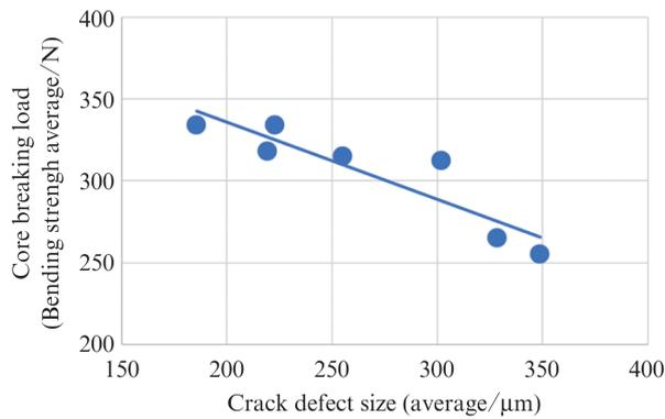
Fig. 8 Effect of crack defect size on core breaking load
