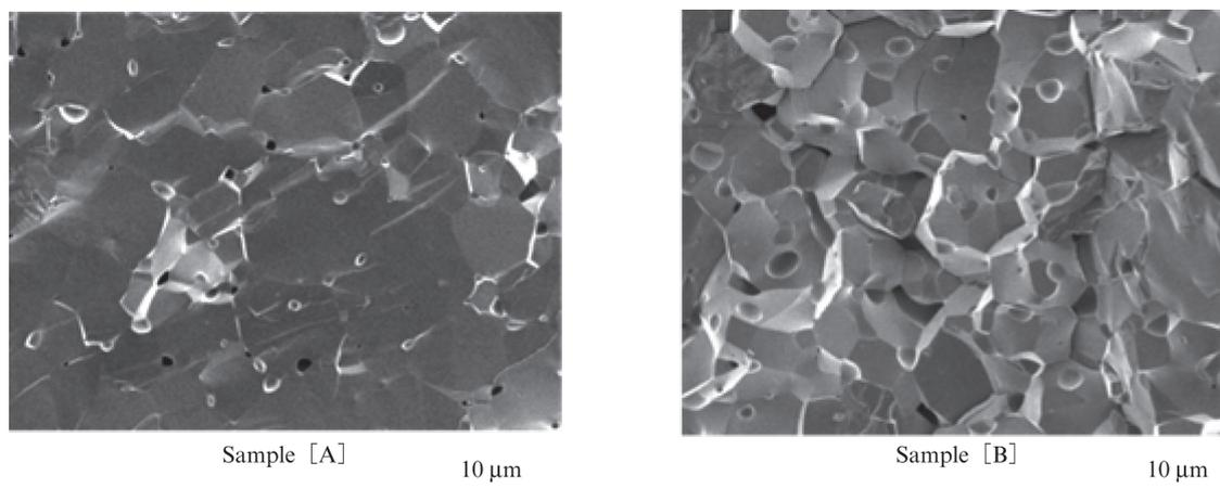
Fig. 6 Comparison of SEM images of fracture surfaces
