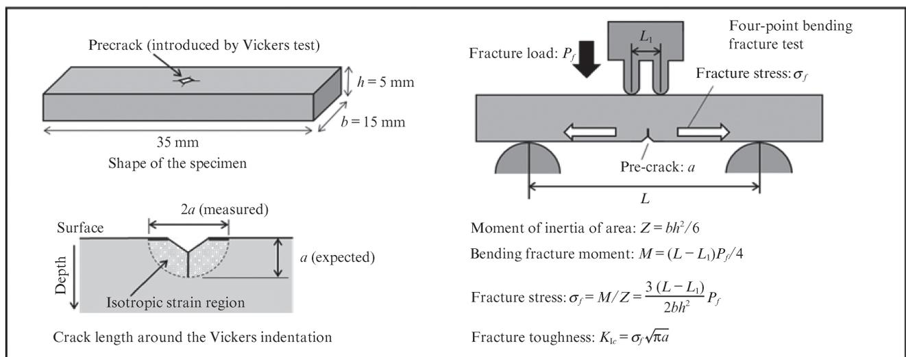
Fig. 3 Schematic diagram of evaluating toughness by Bridge Indentation (BI) method
