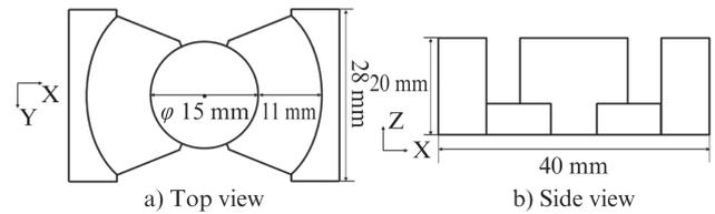
Fig. 2 Top view and side view of ERX40 shape of ferrite core
