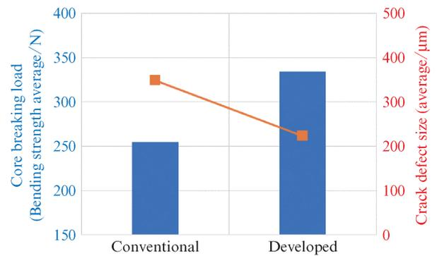
Fig. 9 Effect of higher strength by increasing toughness and suppressing crack defect size
