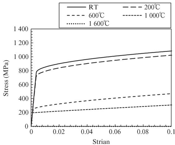
Fig. 4 Examples of stress-strain curves for FEM analysis
