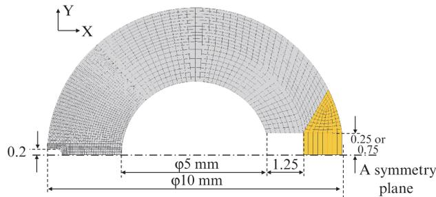
Fig. 3 FEM mesh model of C-ring test specimen
