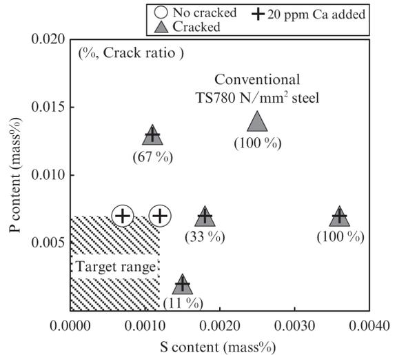
Fig. 8 Effect of P and S content, Ca addition on reheat cracking susceptibility
