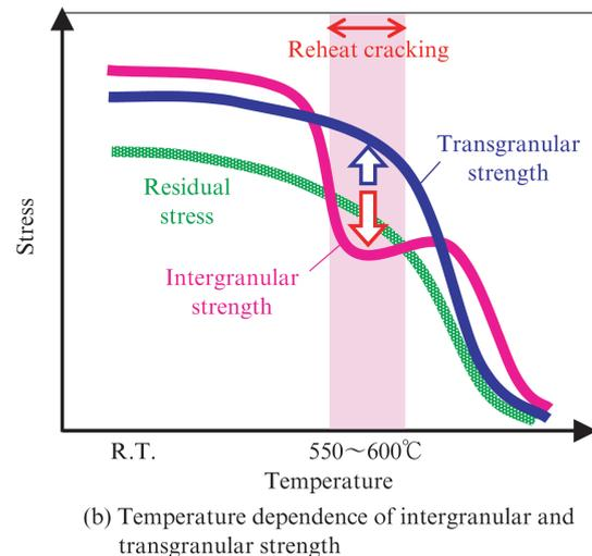
Fig. 1 Schematic illustration of mechanism for reheat cracking
