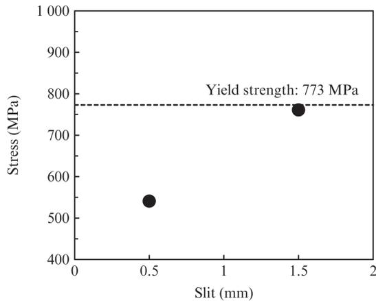
Fig. 7 Effect of slit width on maximum equivalent stress in C-ring specimen
