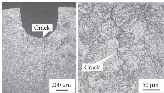
Photo 2 Cross section of C-ring specimen for conventional steel (Notch position: CGHAZ)
