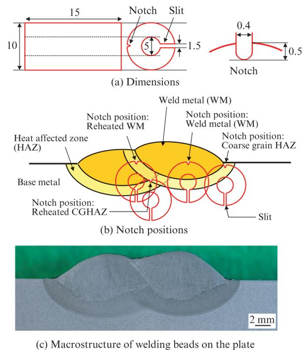
Fig. 2 C-ring test specimen
