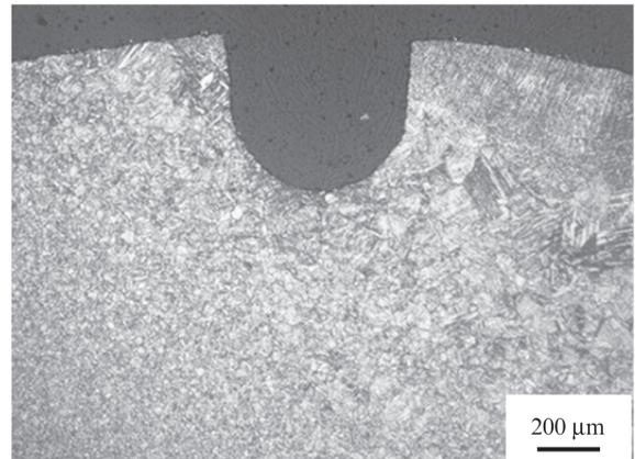
Photo 3 Cross section of notch bottom of C-ring specimens for 0.007% P-0.0012% S-0.0020% Ca steel
