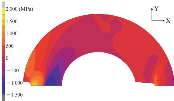
Fig. 6 Principal stress distribution of C-ring test specimen in Y direction
