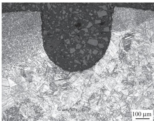
Photo 4 Cross section of notch bottom of C-ring specimens after test for developed steel
