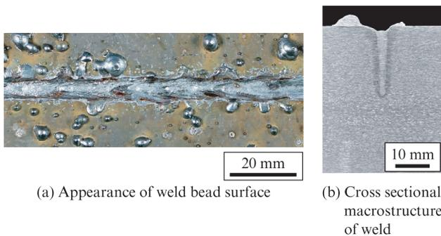
Photo 1 Example of high-power fiber laser welding (Laser power: 25 kW, Welding speed: 1 m/min, Melt run)
