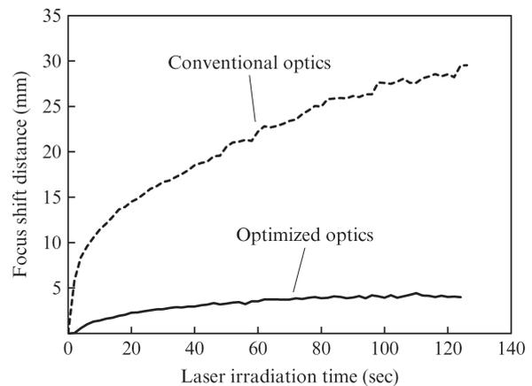
Fig. 5 Comparison of laser beam focus shift distance between before and after optimization of focusing optics
