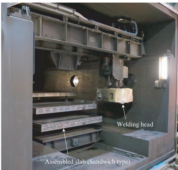
Photo 4 Entrance of vacuum chamber of clad slab assembly line
