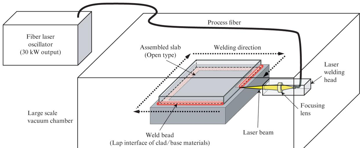
Fig. 7 Schematic illustration of vacuum laser welding system for clad slab assembly
