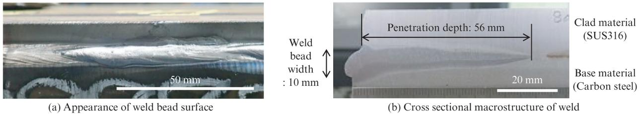
Photo 5 Examples of weld bead appearance and cross sectional macrostructure of vacuum laser weld in clad slab assembly (Laser power: 30 kW, Welding speed: 0.5 m/min)
