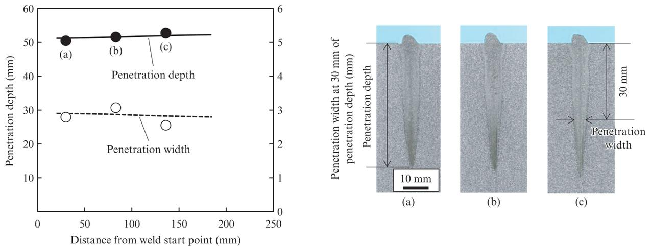
Fig. 6 Penetration shape change with elapsed welding time after optimization of focusing optics (Atmospheric pressure: 100 Pa, Laser power: 30 kW, Welding speed: 0.5 m/min, Melt run)
