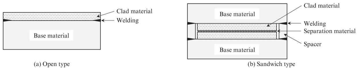
Fig. 3 Slab assembly types of hot rolled clad steel production
