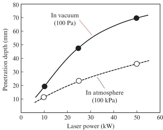
Fig. 1 Comparison of penetration depth of laser welding between in atmosphere and in vacuum (Welding speed: 0.5 m/min, Melt run)
