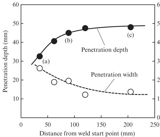
Fig. 4 Penetration shape change with elapsed welding time
