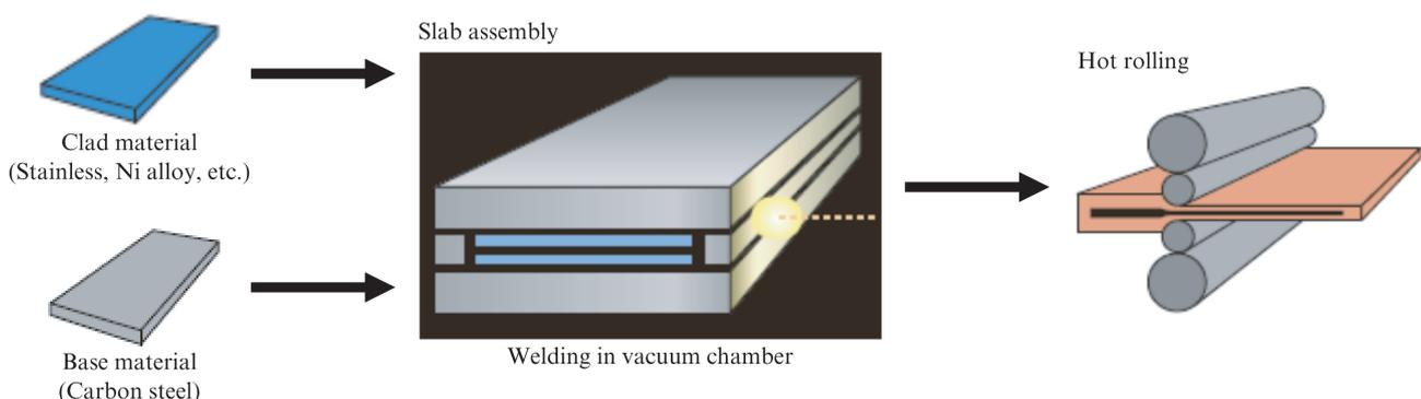
Fig. 2 Outline of production process of hot rolled clad steel
