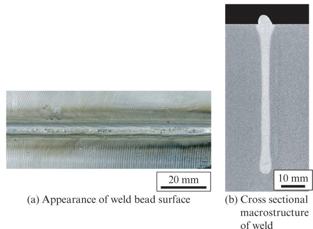
Photo 3 Example of high-power fiber laser welding in vacuum (Atmospheric pressure: 100 Pa, Laser power: 25 kW, Welding speed: 0.5 m/min, Melt run)
