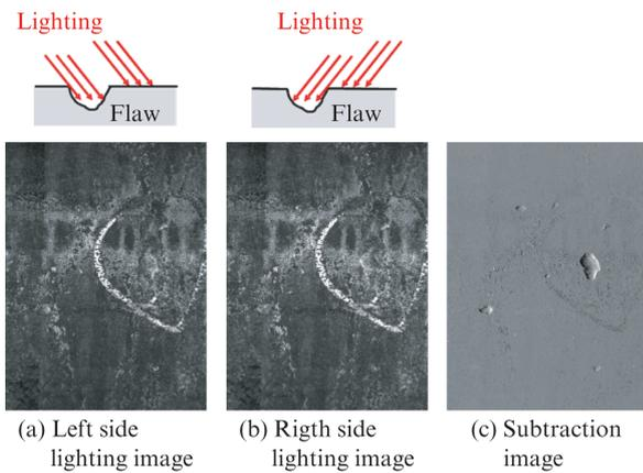
Fig. 6 Effect of developed technique
