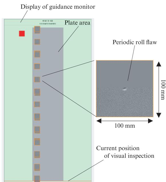
Fig. 8 Guidance monitor of automatic surface inspection system
