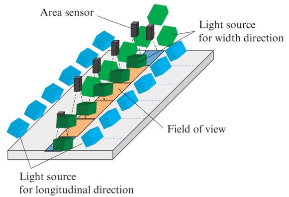
Fig. 7 Overview of automatic surface inspection system for steel plate
