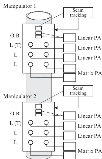
Fig. 1 System configuration of automatic ultrasonic tester
