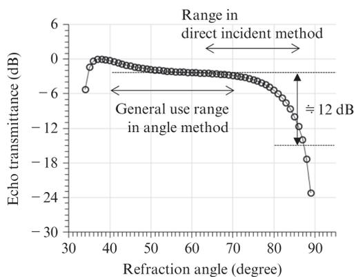
Fig. 2 Relation between refraction angle and echo transmittance
