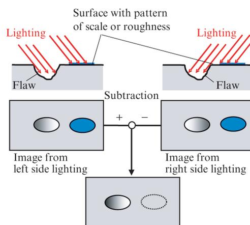
Fig. 5 Principle of twin-illumination and subtraction technique
