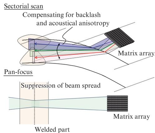
Fig. 3 Direct incident method at the center of wall thickness of welded part using matrix array probe
