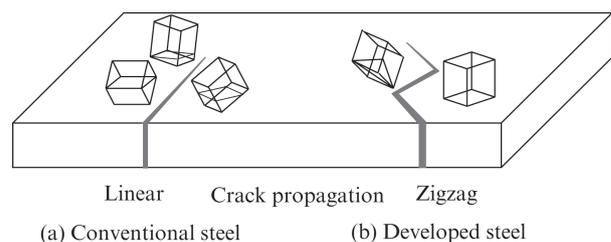
Fig. 2 Concept of improving brittle crack arrestability by texture control
