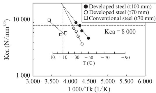
Fig. 3 Results of temperature gradient type standard ESSO test
