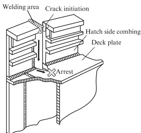
Fig. 1 Container ship superstructure and concept of brittle crack arrest design
