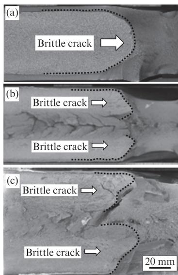
Photo 2 Comparison of fracture appearance of temperature gradient ESSO specimens
