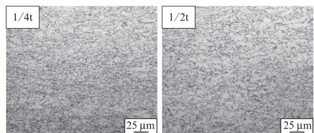
Photo 1 Microstructures of developed steel plate
