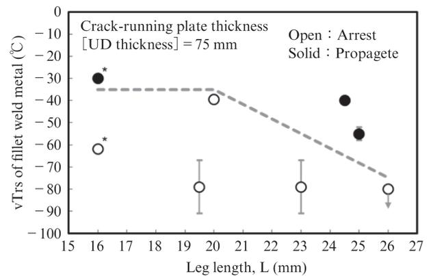
Fig. 9 Relationship between leg length and vTrs of fillet weld metal and long brittle crack propagation/arrest [UD thickness: 75 mm, applied stress: 243 N/mm<sup>2</sup> (\*: 257 N/mm<sup>2</sup>), test temperature: -10°C]
