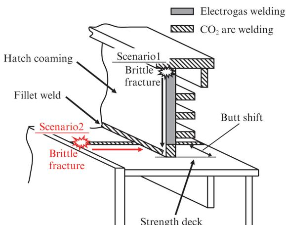
Fig. 1 Brittle crack propagation assumed in this research
