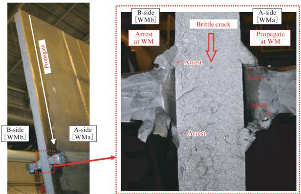
Fig. 6 Fracture surface of ultra-large construction model test specimen [Test 4 (HSC = 60 mmt, UD = 60 mmt)]
