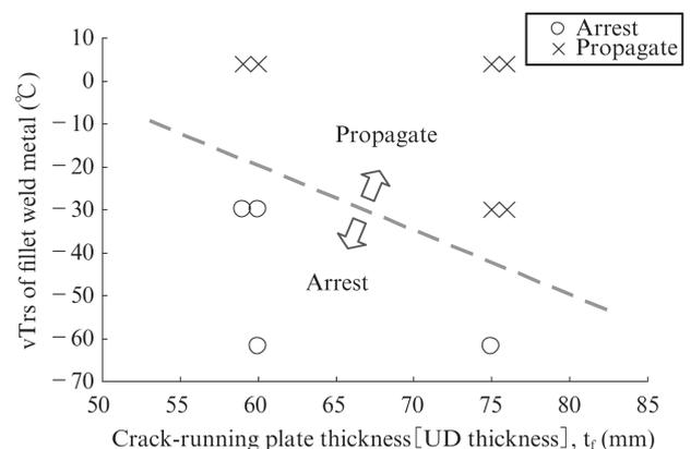
Fig. 7 Relationship between crack-running plate thickness and  $v\text{Trs}$  of fillet weld metal and long brittle crack propagation/arrest [leg length: 16 mm, applied stress:  $257\text{ N/mm}^2$ , test temperature:  $-10^{\circ}\text{C}$ ]
