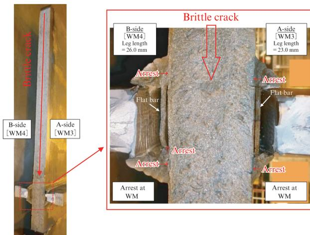
Fig. 8 Fracture surface of ultra-large construction model test specimen [Test 9]
