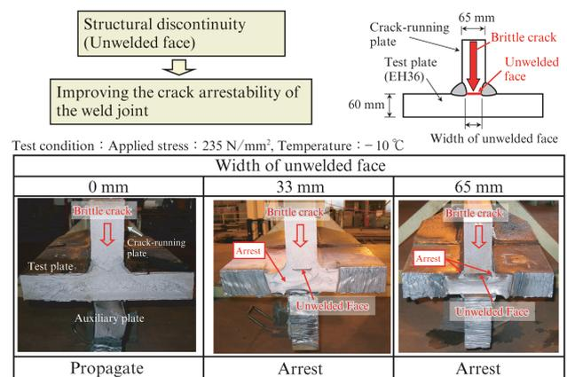
Fig. 2 Effect of structural discontinuity on brittle crack propagation/arrest behavior in Tee joint
