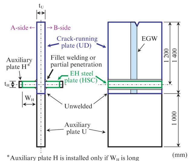
Fig. 4 Dimension of ultra-large construction model test specimens
