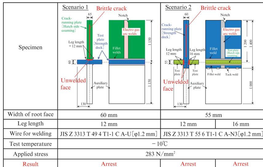
Fig. 3 Results of ultra-large construction model tests
