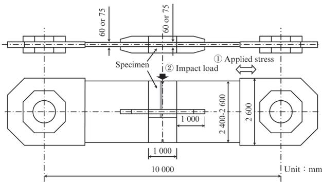
Fig. 5 Dimension of ultra-large construction model tests
