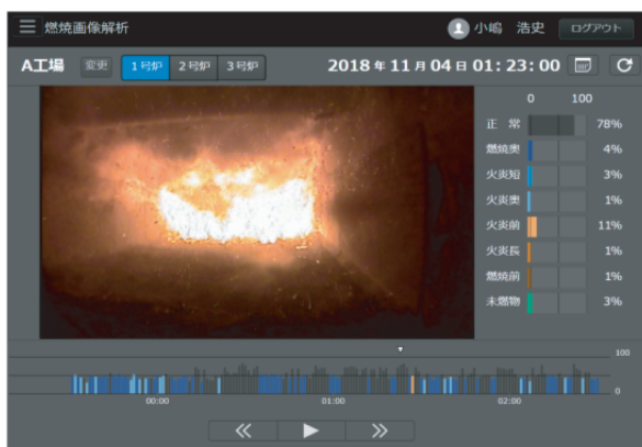
Fig. 7 Visualization monitoring screen of combustion condition analysis system 2, 3)
