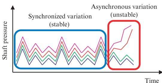
Fig. 10 Normal/Abnormal change of shaft pressure
