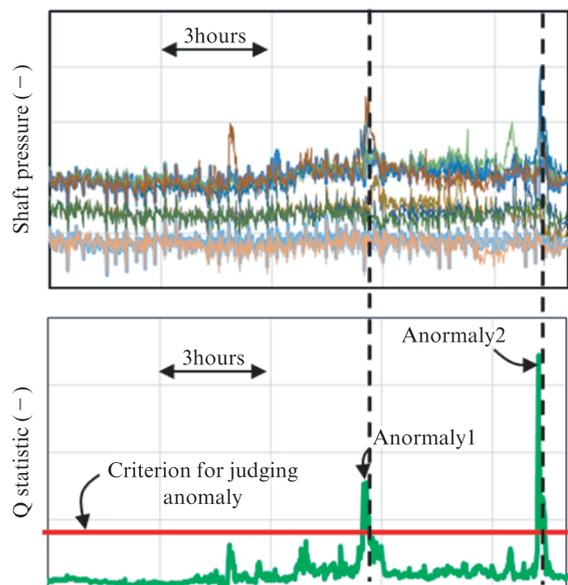
Fig. 12 Example of anomaly detection by Q statistics (Top: Shaft pressure data, Bottom: Q statistics data)
