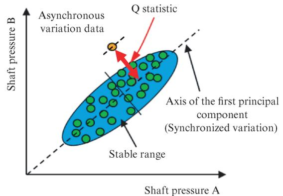
Fig. 11 Anomaly detection of shaft pressure using Q statistics (Example of using only two shaft pressure data)
