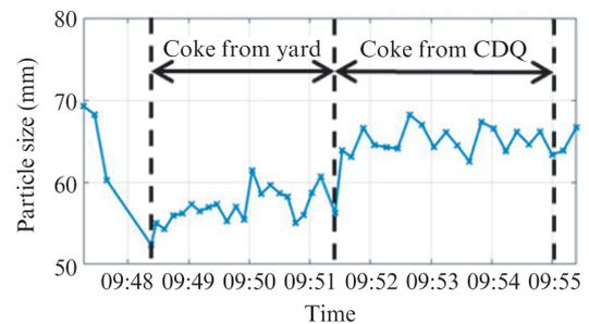
Fig. 4 Result of measurement by particle size meter
