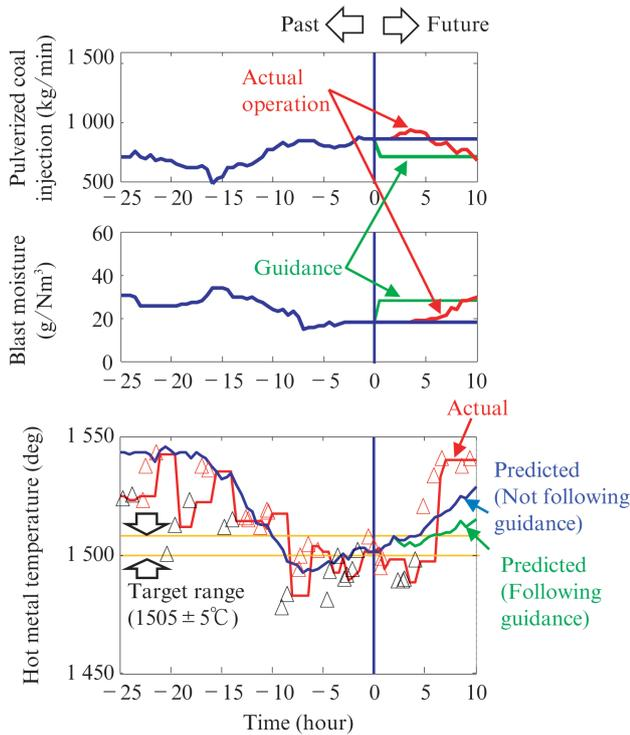
Fig. 7 Predicted hot metal temperature using 2D transient model (Comparison between guidance and actual operation)
