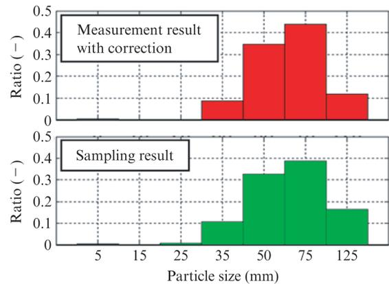
Fig. 3 Comparison of results of measurement by particle size meter and manual analysis by human
