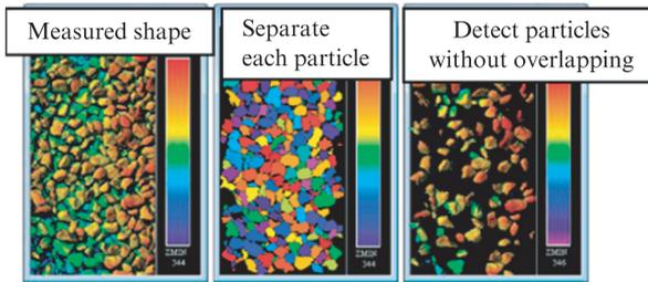
Fig. 2 Schematic diagram of algorithm for calculation of particle size
