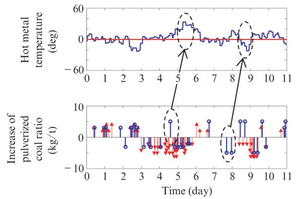
Fig. 8 Result of operation guidance (○ actual operation, △ guidance)
