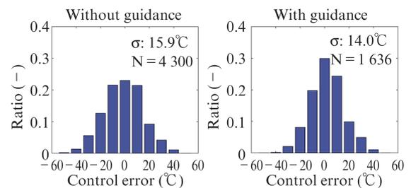
Fig. 9 Control accuracy of hot metal temperature
