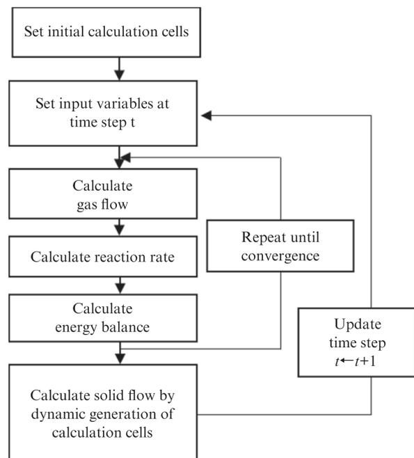
Fig. 6 Flowchart of 2D transient model
