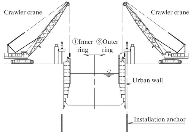
Fig. 9 Assembly of ring pieces
