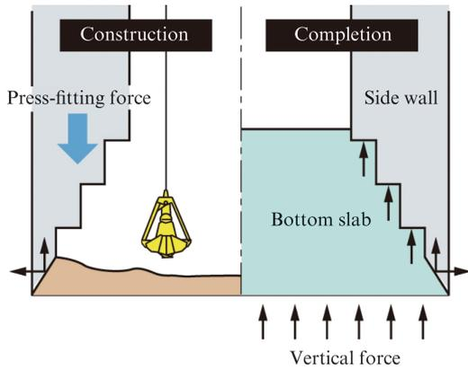
Fig. 8 Cutting edge structure
