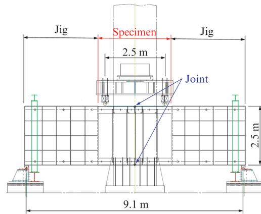
Fig. 12 1/1 scale bending test of the joint
