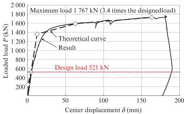
Fig. 11 1/2 scale bending test result of the body
