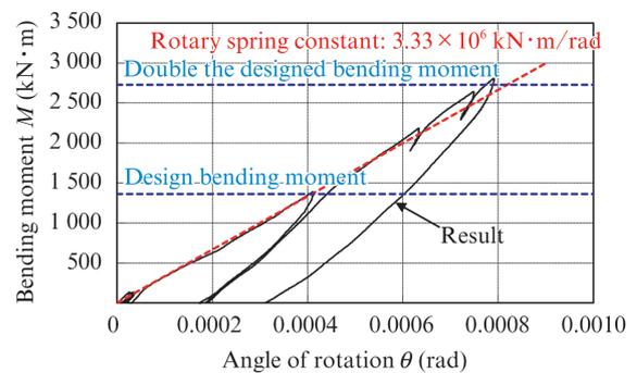
Fig. 13 1/1 scale bending test result of the joint
