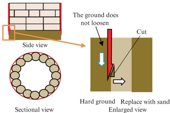
Fig. 5 Mechanism of preceding drilling and cutting edge
