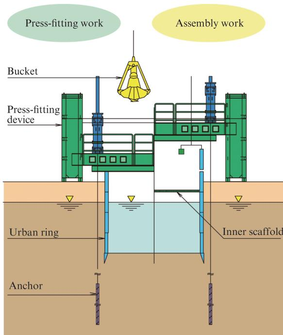
Fig. 2 Drilling Urban-Ring Method™
