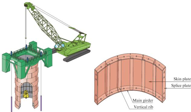
Fig. 1 Steel piece structure
