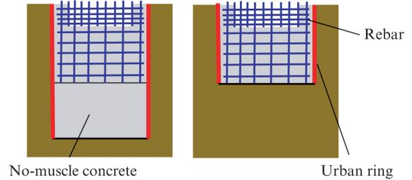
Fig. 4 Comparison of bottom plate
