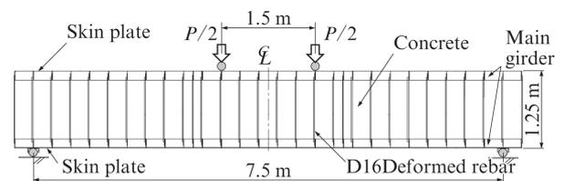
Fig. 10 1/2 scale bending test of the body
