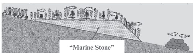
Fig. 1 Cross-sectional image of shoal created using “Marine Stone” in Iwakuni, Yamaguchi Pref. 5)
