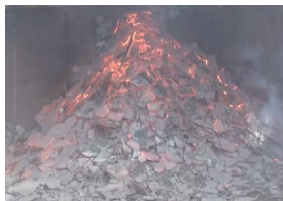
Photo 3 Plate-like solidified slags
