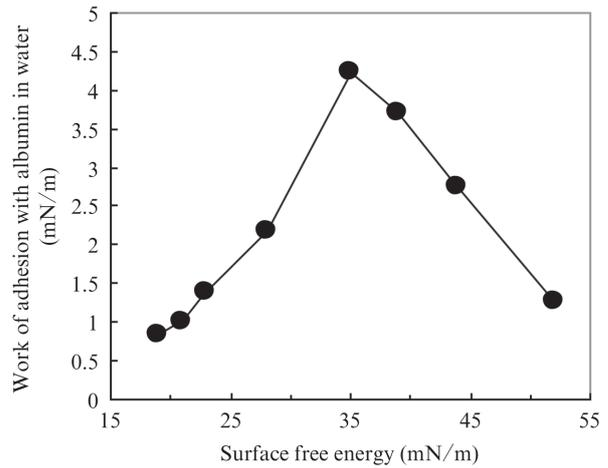
Fig. 5 Relation between surface free energy and work of adhesion with albumin in water
