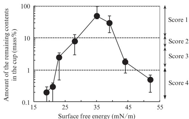
Fig. 3 Effect of surface free energy on content release properties
