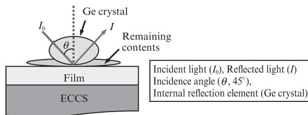
Fig. 2 ATR measurement method
