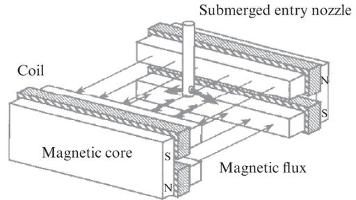
Fig. 8 Schematic drawing of Flow Control Mold
