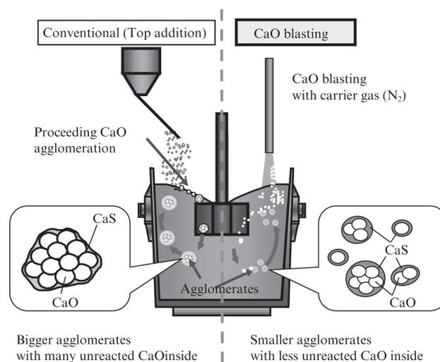
Fig. 3 Comparison of conventional and developed method in hot metal desulfurization with mechanical stirring
