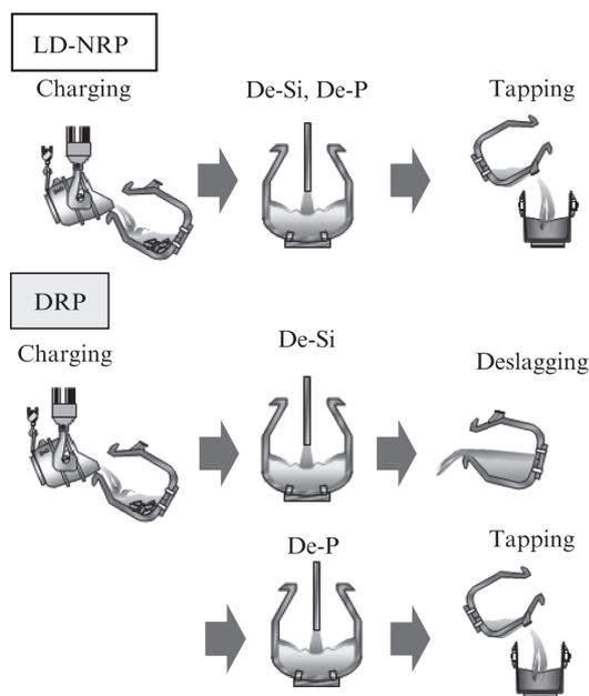
Fig. 2 Schematic image of new hot metal dephosphorization process using converter (DRP<sup>®</sup>)
