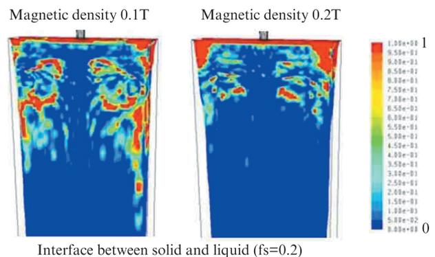
Fig. 9 Calculated results of entrapped bubble concentration
