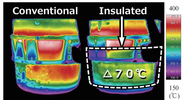
Fig. 5 Comparison of temperature distributions in steel ladles with and without heat insulation
