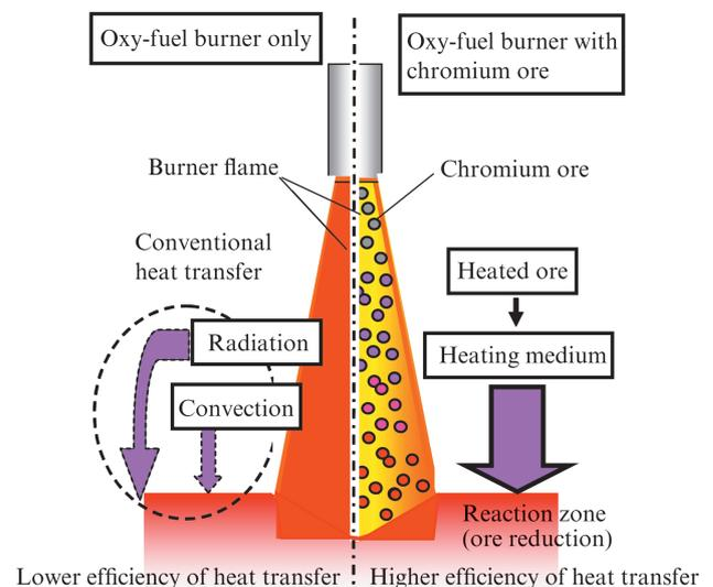
Fig. 6 Comparison of conventional and developed heat transfer
