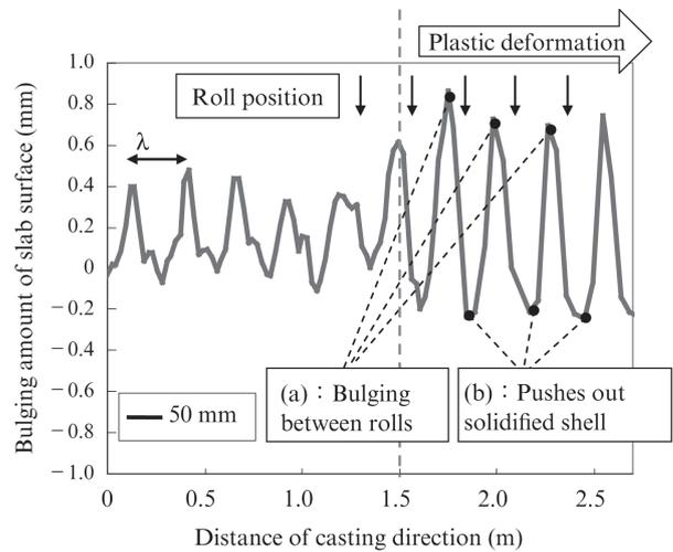
Fig. 13 Bulging amount of slab surface (shell thickness 50 mm)
