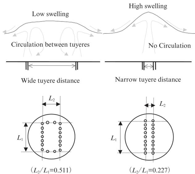
Fig. 4 Observation results of bath flow patterns with different tuyere array distances
