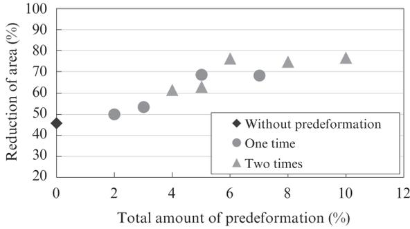
Fig. 10 Improvement of hot ductility by predeformation treatment
