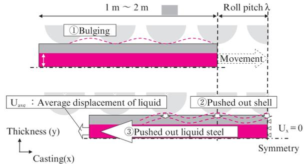
Fig. 12 Schematic drawing of displacement of liquid in elasto-plastic analysis
