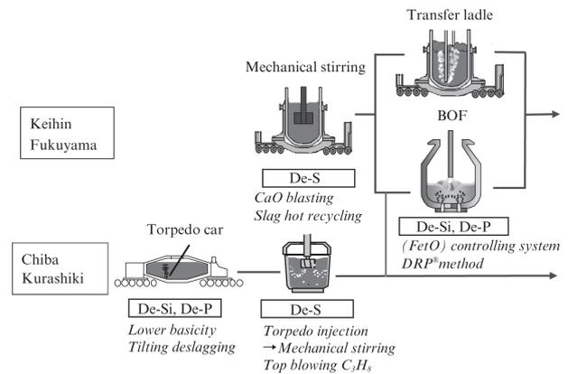
Fig. 1 Developed techniques in hot metal pretreatment process
