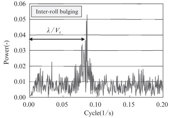
Fig. 11 FFT analysis of inter-roll bulging fluctuation
