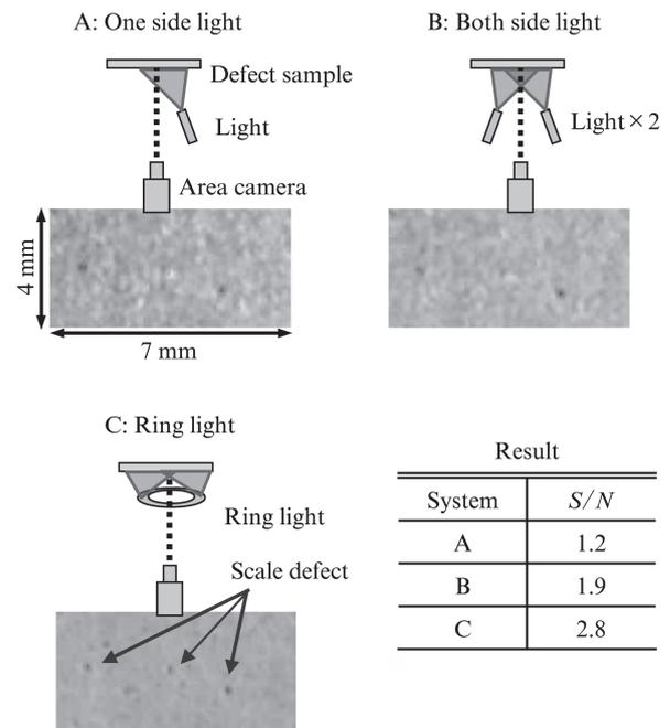
Fig. 2 Results of scale defect imaging tests
