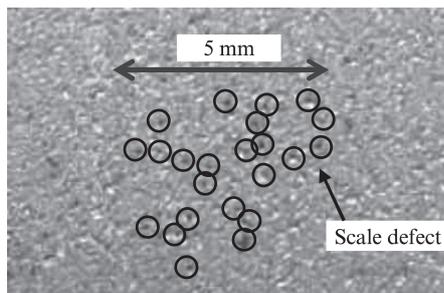
Photo 1 Example of the scale defect
