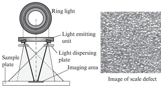
Fig. 3 Result of scale defect imaging tests applying standard ring light unit
