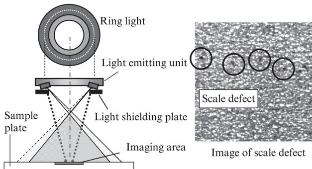
Fig. 4 Result of scale defect imaging tests applying improved ring light unit
