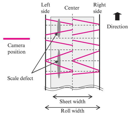
Fig. 6 Inspection area on steel sheet
