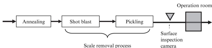
Fig. 1 Stainless steel manufacturing process
