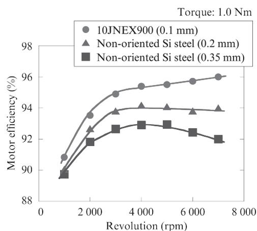
Fig. 7 Motor efficiency and motor speed<sup>4)</sup>
