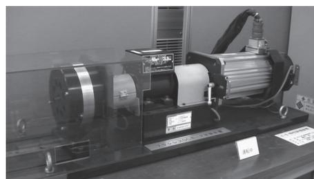
Photo 3 Model motor evaluation system
