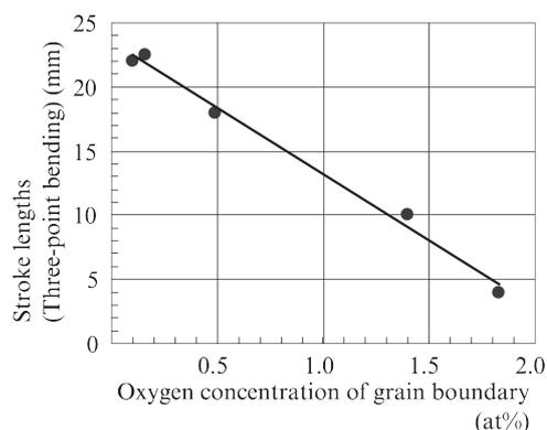
Fig. 6 Result of three-point bending test
