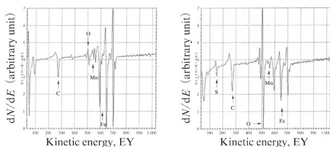
Fig. 5 Analysis of grain boundary
