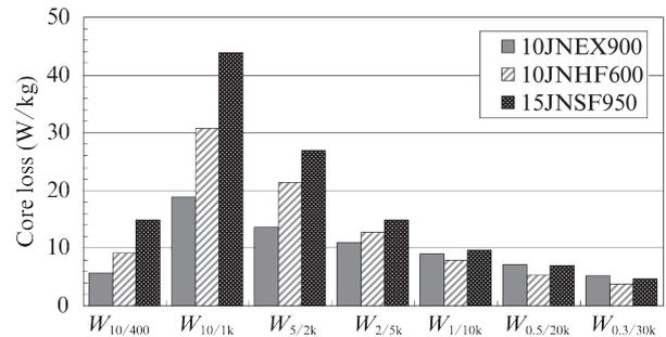
Fig. 4 Core losses of “JNEX™,” “JNHF™,” and “JNSF™”
