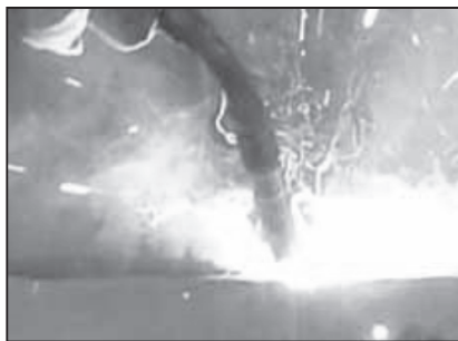
(a) Conventional welding; DCEP (Direct current electrode positive), Welding current: 280 A
