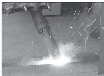
(b) “J-STAR™ Welding”; KC-550, DCEN (Direct current electrode negative), Welding current: 380 A
