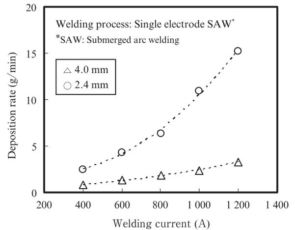
Fig. 3 Effect of welding wire diameter on deposition rate
