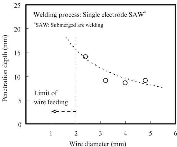
Fig. 4 Effect of wire diameter on penetration depth
