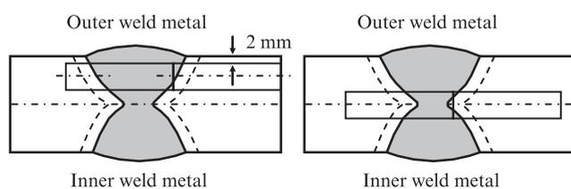
Fig. 6 Charpy V-notch impact test specimen positions
