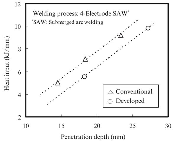
Fig. 5 Heat input reduction effect on 4-electrode SAW
