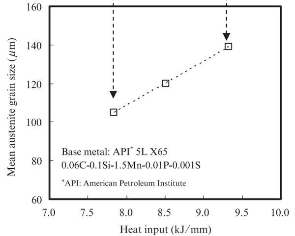
Fig. 2 Effect of heat input of double submerged arc welding (DSAW) on austenite grain size
