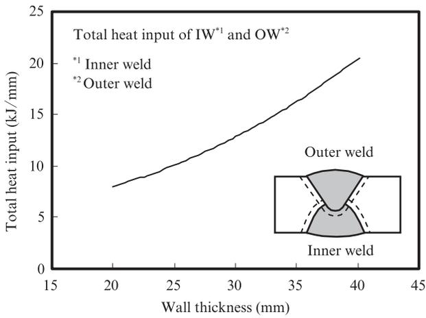
Fig. 1 Relationship between wall thickness and heat input on seam welded joint on UOE linepipe
