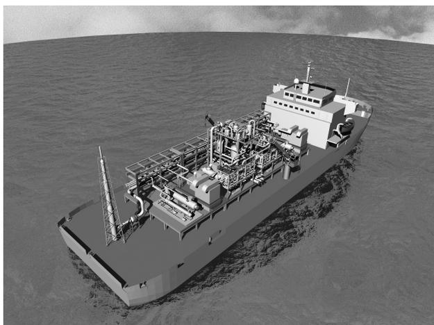
Fig. 2 Custom build vessel for offshore tanker vapor recovery (TVR)
