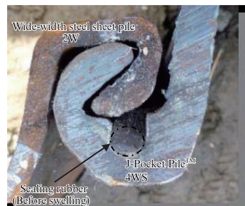
Photo 3 Fitting condition between 4WS and 2W
