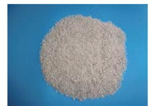
(6) No. 6 Granulated blast furnace slag
