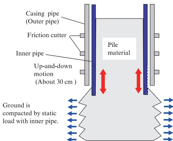
Fig. 1 Casing with a double pipe (Geo-KONG method)
