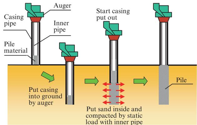
Fig. 2 Construction procedure of Geo-KONG method
