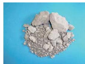
(5) No. 5 Artificial stone made by steel slag
