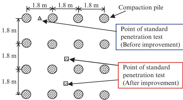
Fig. 6 Arrangement of sand compaction pile
