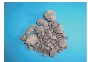
(4) No. 4 Converter slag (Unaged)
