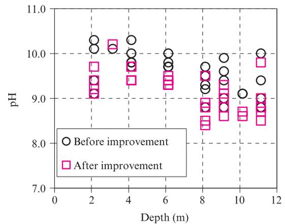
Fig. 9 pH Measured in each depth
