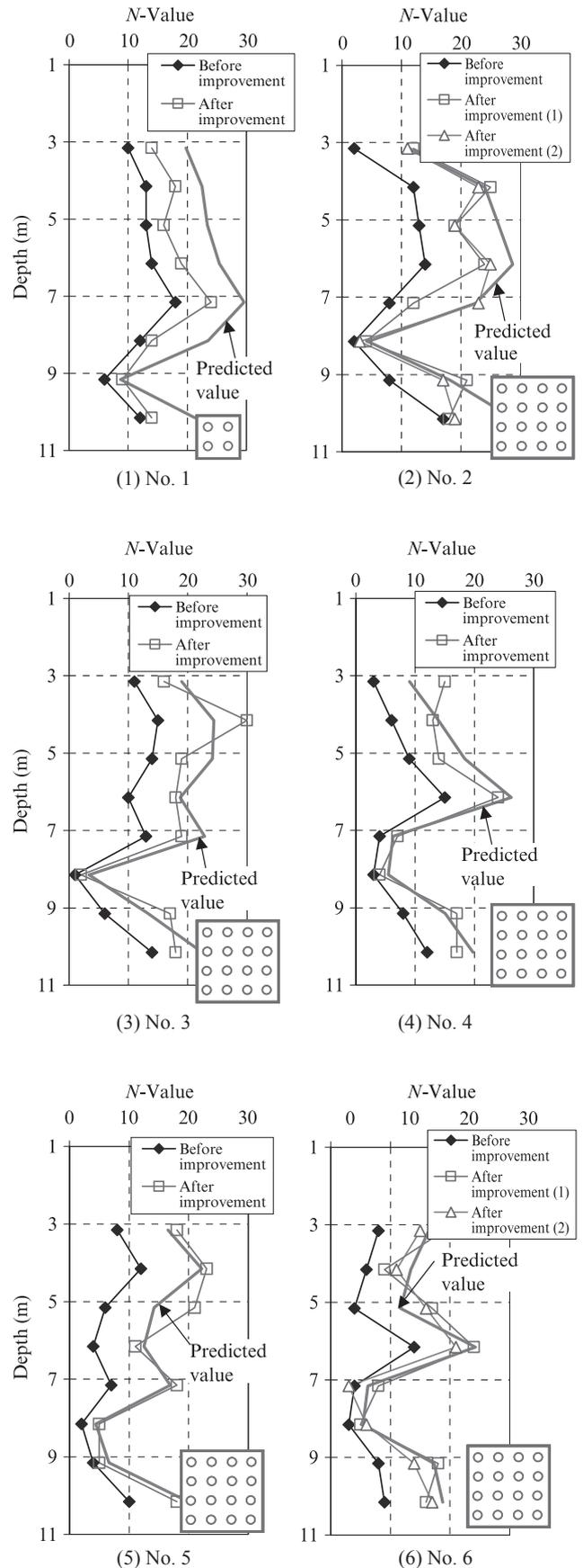
Fig. 7 Increased penetration resistances in ground improved by the Sand Compaction Pile method
