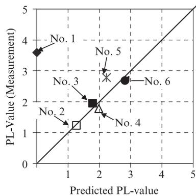
Fig. 8 Comparison of predicted liquefaction index (PL)-value and measured PL-value
