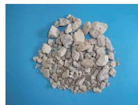
(3) No. 3 Air-cooled blast furnace slag
