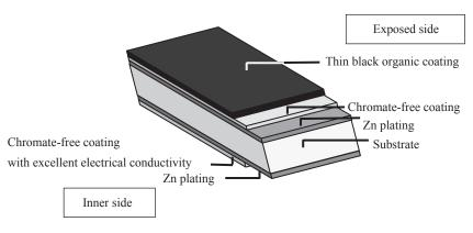
Fig. 1 The coating structure of ECO-BLACK<sup>™</sup>
