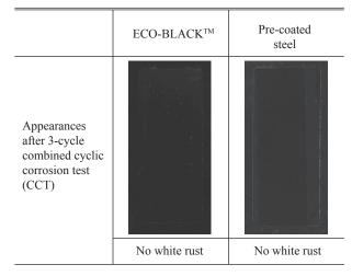
Photo 3 Corrosion resistance of ECO-BLACK<sup>™</sup>
