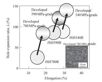
Fig. 1 Balance of elongation and hole-expansion ratio
