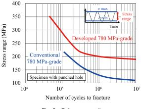
Fig. 2 Fatigue properties
