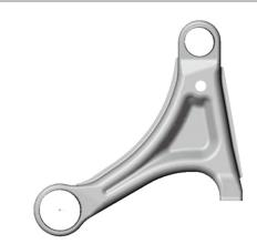
Fig. 3 Application of developed 780 MPa-grade steel to lower-arm
