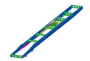
Fig. 4 Application of developed 780 MPa-grade steel to truck frame
