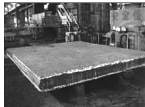
Photo 1 Forged slab using ingot (Removed surface scale)
