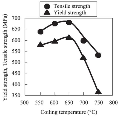
Fig. 4 Effect of coiling temperature on the strength
