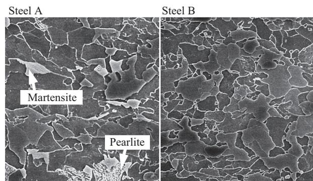
Photo 2 Effect of carbon on the microstructure
