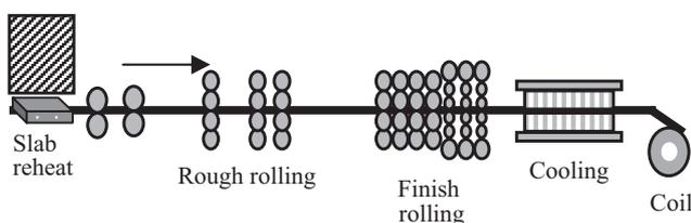
Fig. 1 Hot rolling process
