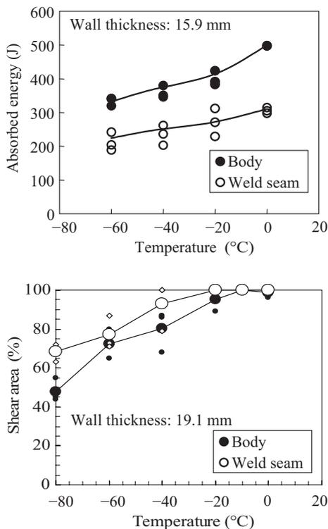
Fig. 7 Charpy V notch test results
