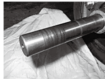
Photo 1 Shaft photograph after burning examination ends
