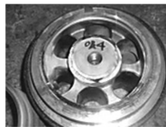
Photo 2 Detached inhalation valve (loss on seat side)
