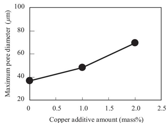
Fig. 8 Maximum pore size of the sintered and case-hardened compacts made of the low molybdenum prealloyed steel powder with copper addition
