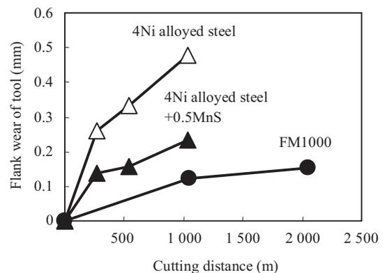
Fig. 5 Machinability of the sintered compacts made of FM1000 and the 4Ni alloyed steel powder mixture
