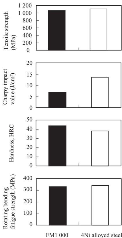
Fig. 4 Mechanical properties of the sintered and case-hardened compacts made of FM1000 and the 4Ni alloyed steel powder mixture
