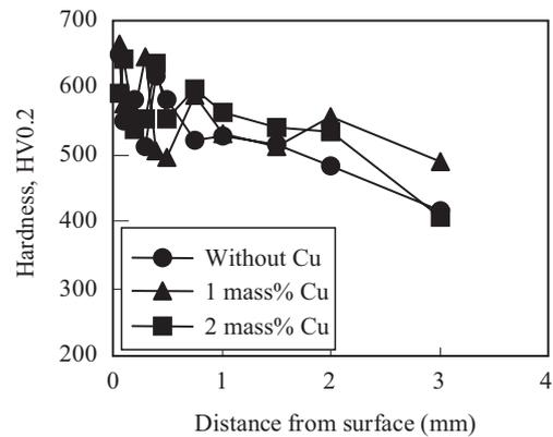
Fig. 7 Microhardness profiles in the surface layer of the sintered and case-hardened compacts made of the low molybdenum prealloyed steel powder with copper addition
