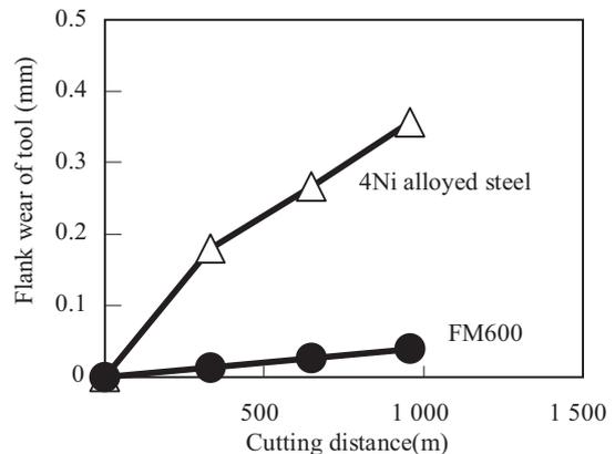
Fig. 3 Machinability of the sintered compacts made of FM600 and the 4Ni alloyed steel powder mixture
