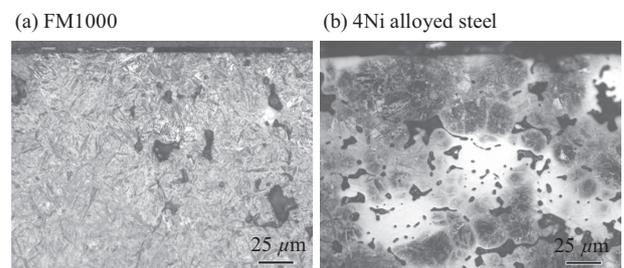
Photo 3 Microstructures of the sintered and case-hardened compacts made of FM1000 (a) and the 4Ni alloyed steel powder mixture (b)
