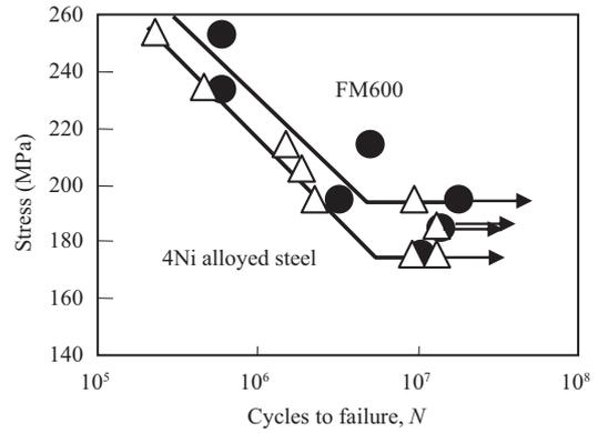
Fig. 2 Results of rotating bending fatigue tests of the sintered compacts made of FM600 and the 4Ni alloyed steel powder mixture
