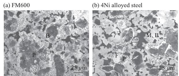
Photo 1 Microstructures of the sintered compacts made of FM600 (a) and the 4Ni alloyed steel powder mixture (b)
