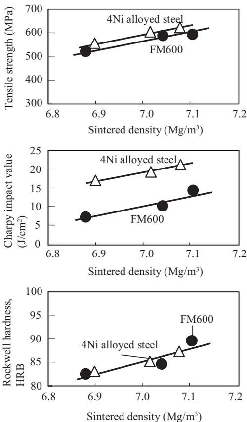
Fig. 1 Mechanical properties of the sintered compacts made of FM600 and the 4Ni alloyed steel powder mixture
