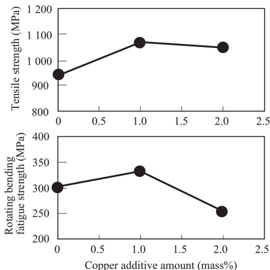
Fig. 6 Effects of copper addition on mechanical properties of the sintered and case-hardened compacts made of the low molybdenum prealloyed steel powder
