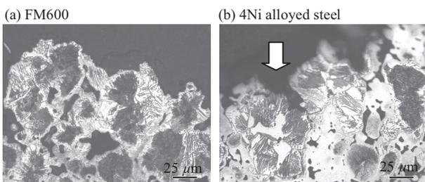
Photo 2 Fatigue crack propagation path observed at the cross-section of fatigue fracture surfaces of the sintered compacts made of FM600 (a) and the 4Ni alloyed steel powder mixture (b)
