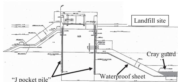
Fig. 7 Cross section of seawall
