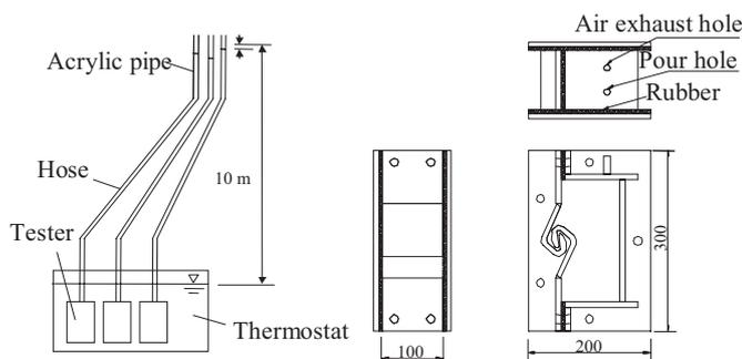
Fig. 1 Test equipment
