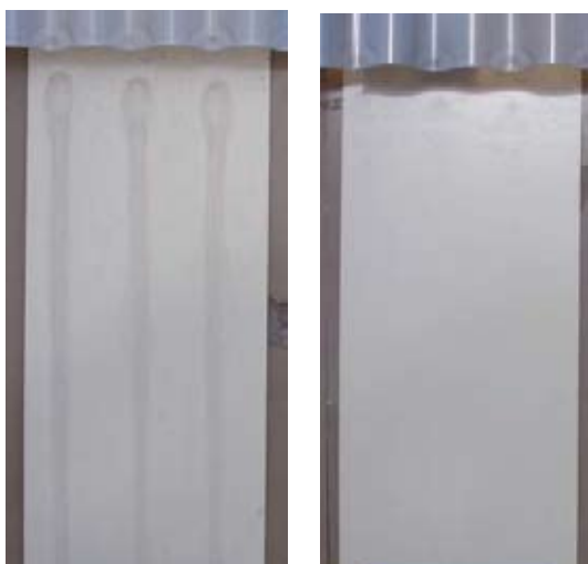
Conventional pre-painted steel New type of pre-painted steel
