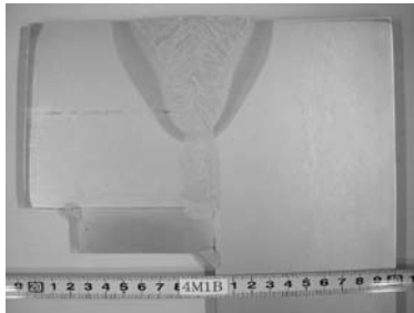
Photo 6 Macroetch test specimen for corner welding
