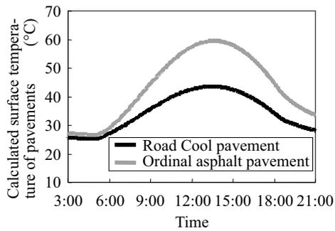
Fig. 7 Calculated surface temperature of Road Cool pavement and ordinal asphalt pavement
