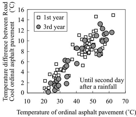
Fig.6 Temperature difference between Road Cool pavement and ordinal asphalt pavement
