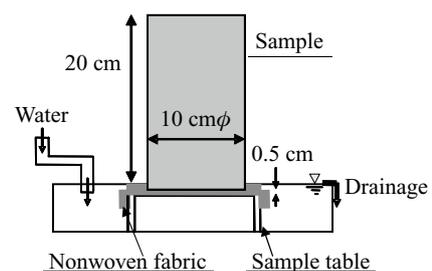
Fig. 1 Schematic diagram of water absorbing test
