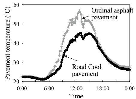
Fig.5 Typical results of surface temperature of Road Cool pavement and ordinal asphalt pavement at third summer
