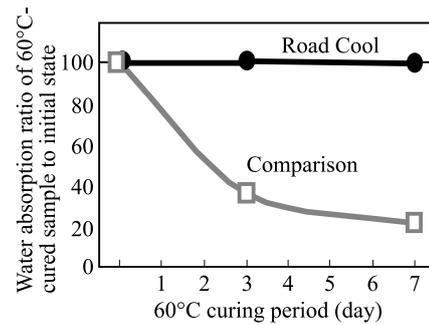
Fig.4 24-hour water absorption of 60°C-cured water retentive materials after various curing period
