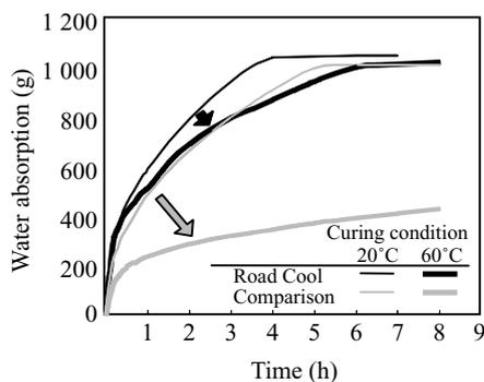
Fig.3 Water absorption of water retentive materials after 20°C and 60°C during
