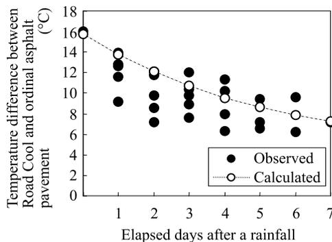
Fig. 8 Relationship between elapsed days after a single rainfall and reduced surface temperature by using Road Cool
