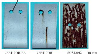
Photo 2 Appearance of salt spray test specimens (testing time; 96 h) in JFE410DB-ER, JFE410DB, and SUS420J2.
