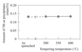
Fig. 5 Amount of Nb as precipitates in Steel B(Nb added) tempered at each temperature for 60 min.
