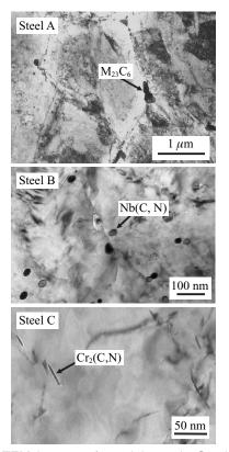
Photo 1 TEM images of precipitates in Steel A(base), B(Nb added), and C(high N) tempered at 550°C for 60 min
