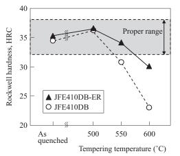
Fig. 8 Change in hardness with tempering temperaturein JFE410DB-ER and JFE410DB
