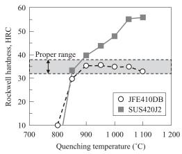
Fig.2 Quenching hardenability in JFE410DB and SUS420J2 (Specimens were quenched by air cooling after holding at each temperature for 10 min.)
