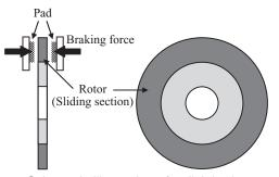
Fig. 1 Schematic illustration of a disk brake system
