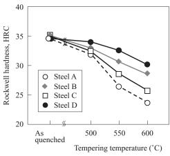
Fig. 3 Effects of Nb and N on temper softening
