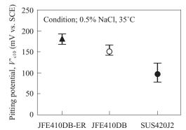
Fig. 10 Pitting potential in JFE410DB-ER and JFE410DB (Specimens were quenched from 1 000°C.)
