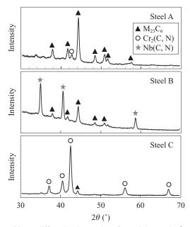
Fig. 4 X-ray diffraction intensity of precipitates in Steel A (base), B(Nb added), and C(high N) tempered at 550°C
