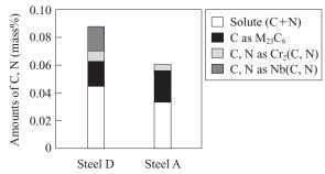
Fig.6 Amount of solute/precipitated C, N in Steel A(base), and D(Nb + high N) tempered at 550°C
