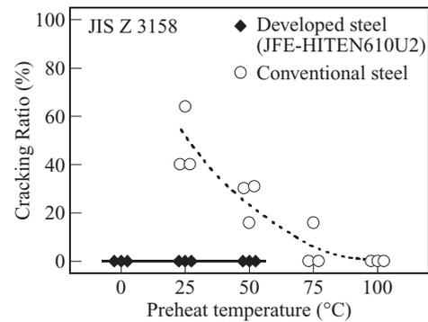
Fig. 7 Decrease of preheat temperature to avoid weld cracking of the developed steel by suppression of C and  $P_{CM}$
