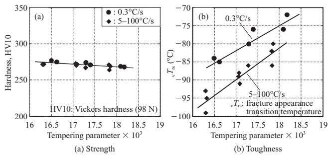
Fig. 6 Relationship between tempering parameter and mechanical properties of 780 MPa class steel
