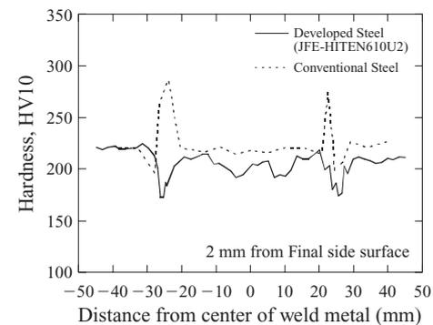
Fig. 8 Improvement of HAZ hardness distribution of the developed steel by suppression of C content and  $P_{CM}$
