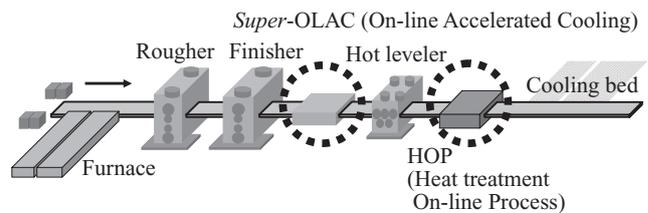
Fig. 2 Layout of online heat-treatment facilities of West Japan Works (Fukuyama)
