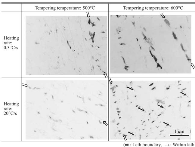
Fig.4 Precipitation behavior of cementite during heating process
