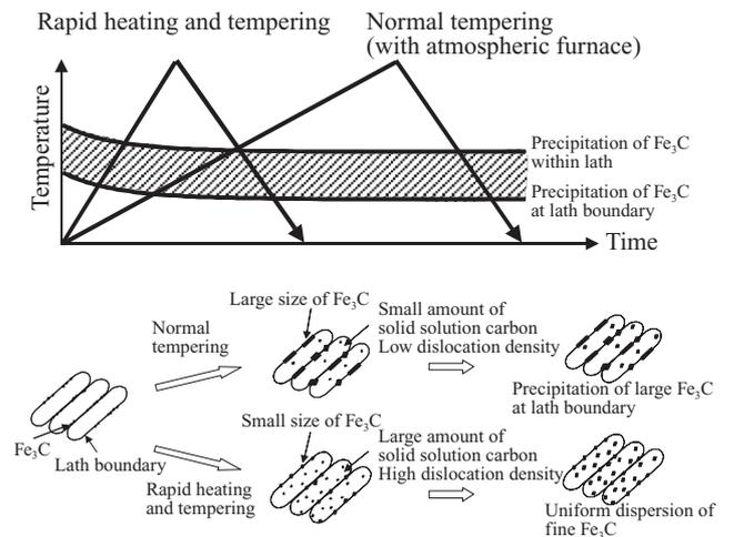
Fig.5 Mechanism of uniform dispersion of fine cementite by rapid heating and tempering
