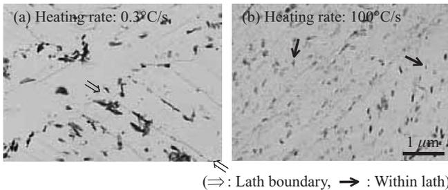
Fig.3 Uniform dispersion of fine cementite by rapid heating and tempering
