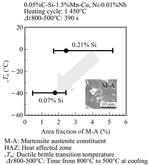
Fig.2 Effect of Si contents on synthetic HAZ toughness
