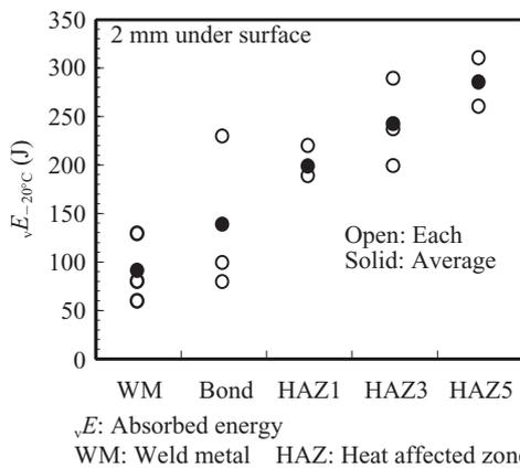
Fig.3 Charpy impact properties of EGW welded joint
