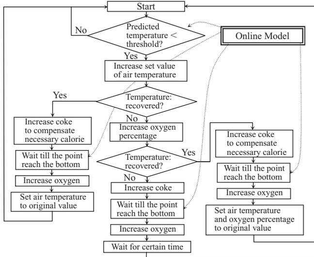
Fig. 7 Rule-based control algorithm with online prediction model
