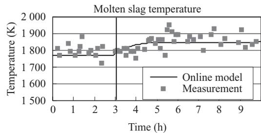
Fig. 6 Comparison between model estimation of molten slag
