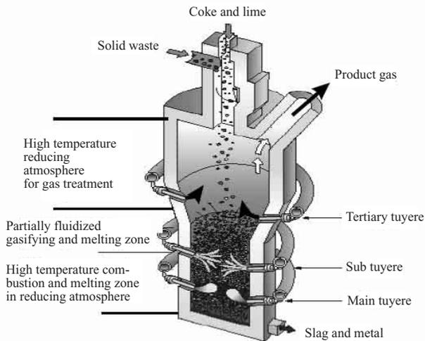
Fig. 1 Schematic diagram of high-temperature gasifying and direct melting furnace
