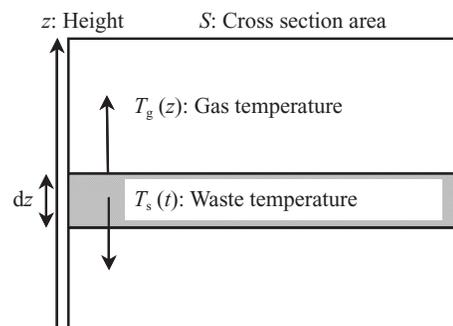
Fig. 4 Heat transfer in countercurrent flow model
