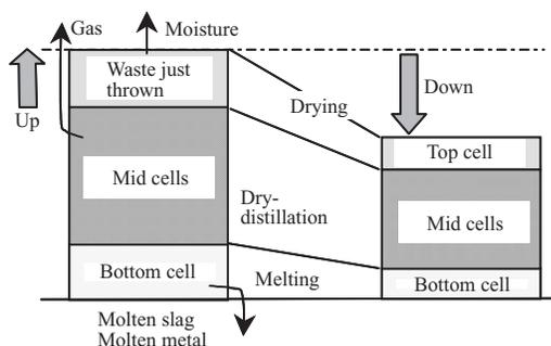
Fig. 3 Conceptual diagram of waste tracking model
