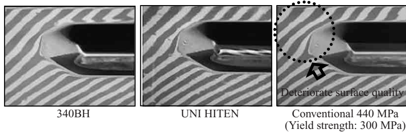
Fig. 6 Comparison between the conventional 440 MPa steel and the 440 MPa grade UNI HITEN on the surface distortion by optical method
