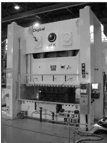
Photo 1 Servo press machine installed JIM-Form technology
