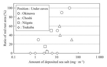
Fig. 2 Relationship between amount of deposited sea salt and corrosion of collected air-conditioners (air vent of side cover)<sup>23,25)</sup>
