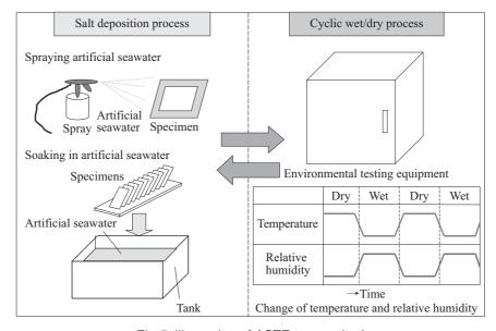
Fig.5 Illustration of ACTE test method
