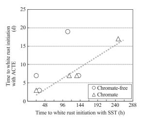
Fig. 7 Comparison of time to white rust initiation with ACTE and SST<sup>24)</sup>
