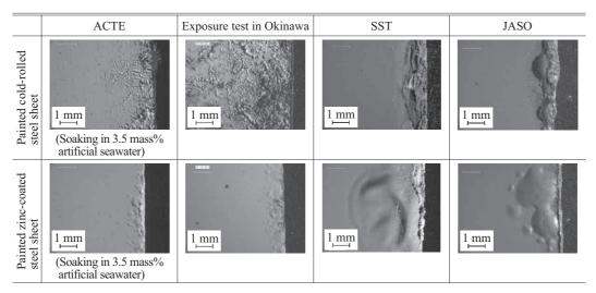
Photo 1 Comparison of corrosion morphology of painted steel sheets
