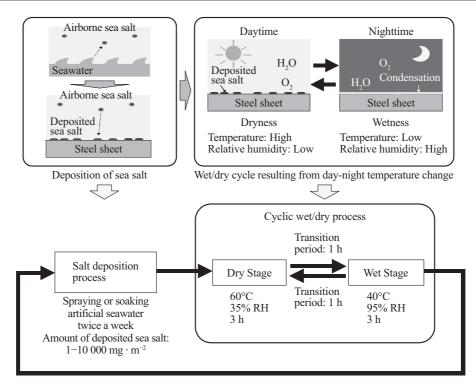
Fig.4 Example of test conditions of new accelerated corrosion test "ACTE"24-28)
