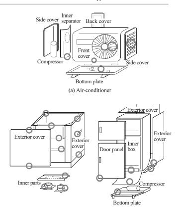
Fig. 1 Location of parts of electrical appliances with high susceptibility to corrosion<sup>19,20)</sup>
